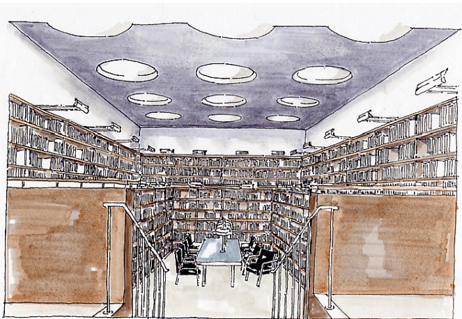
Figure 11. Example of a skylight roof aperture system for a special collections room. Note the architecturally interesting ceiling that results. (Pensions Institute, Special Collection, Helsinki, Finland)
