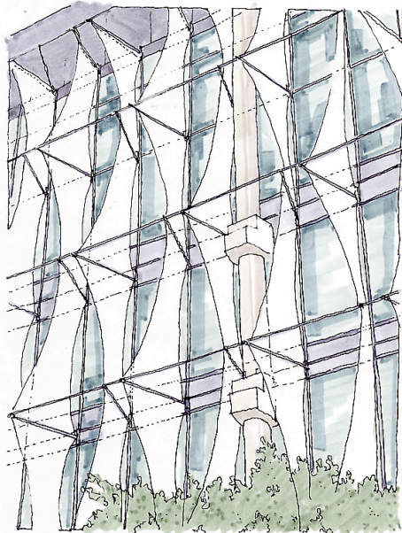
Figure 16. Exterior sunshade for a north-facing glass wall. The design protects against late afternoon mid-summer sun and reduces glare from bright surroundings. (Phoenix Central Library, Phoenix, Arizona)
