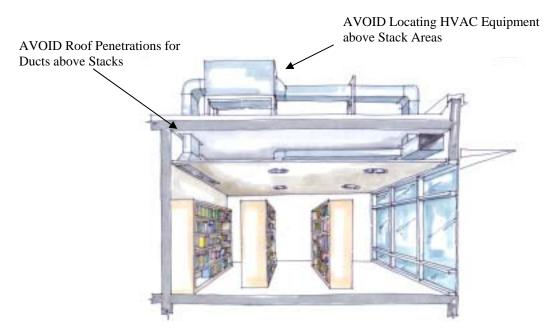
Figure 4. Illustration of Poor HVAC Equipment Siting.
