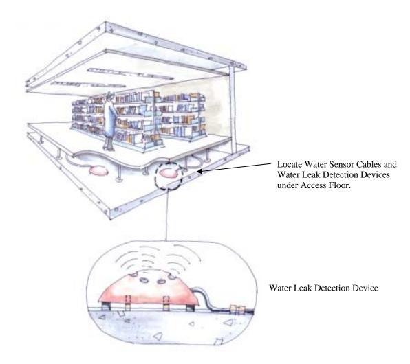
Figure 3. Water Leak Detection under Access Floors
