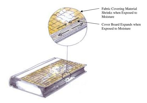
Figure 6. Different Rates of Expansion between Adhered Materials Produce Damage when Exposed to Moisture.
