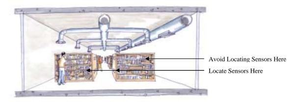
Figure 8. Place System Sensors away from Air Supply Outlets.
