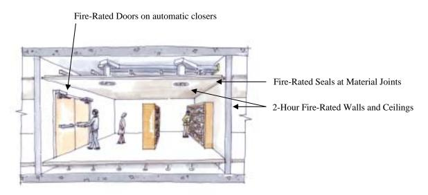
Figure 1. Special Collection Area separated through Compartmentation.
