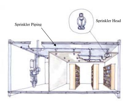
Figure 2. Typical Water Fire Protection System
