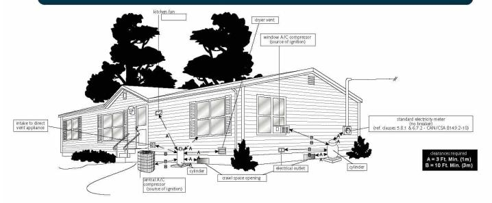
NOTE: Clearance required between cylinder and heat exchanger: 10 ft min. (3 m) from air intake and 3 ft min. (1 m) from air outlet
