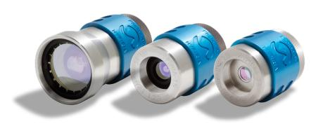
The HypIRia are wide-aperture, image-space telecentric lenses precisely crafted to provide clear and bright images in the SWIR spectral range. A broadband anti-reflective coating on carefully selected glass delivers high throughput and low-aberration imaging on an range extending from 1.0 to  $2.9~\mu m$ .
