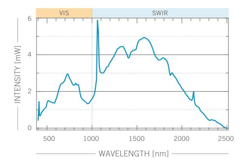
FIG. A3: Output from Photon etc's tunable laser source. Visible option covering 400 - 1000 nm and SWIR option covering 1000 - 2500 nm.
