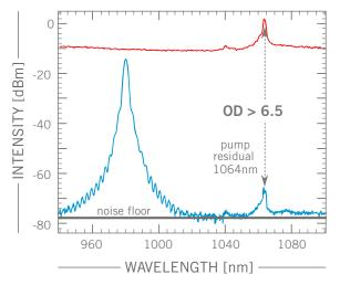
FIG. 5: Measurements of the optical density (OD =  $\log_{10}(I_0/I_t)$ ) at the pump energy (1064 nm). Blue: LLTF Contrast<sup>TM</sup> output (I<sub>t</sub>), Red: unfiltered supercontinuum output (I<sub>0</sub>). Those measurements were realised with the setup shown in FIG. 3.
