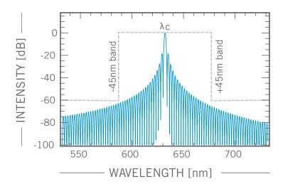
FIG. 1.1: Illustration of the out-of-band rejection of a volume holographic grating at  $\lambda_c = 632$  nm. Bands of ±45 nm are presented and an out-of-band rejection of -60 dB is obtained.
