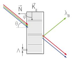
FIG. A1: Schematic of a volume holographic transmission grating.
