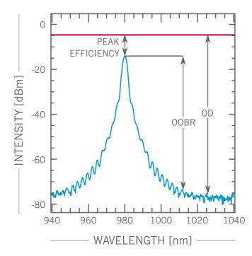
FIG 1.2: Comparison of the concepts of out-of-band-rejection (OOBR), optical density (OD) and filter peak efficiency. Red curve: hypothetical optical source, bleu curve: hypothetical spectral response of the filtered source.
